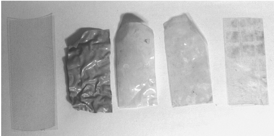
Figure 6 - 8: Changes in PVC-material VI, the packaging foil, caused by the different kinds of treatment; from left to right: 1. raw material, 2. PVC VI from lysimeter 2 (aerobic), 3. PVC VI from lysimeter 4 (aerobic-anaerobic), 4. PVC VI from lysimeter 6 (anaerobic), 5. PVC VI from biological waste treatment plant
